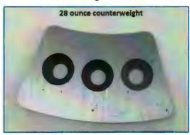
Ensure that the counterweight flywheel bolt holes threads are clean of oil, failure to do so will compromise the thread locker that is applied to the counterweight bolts and may result in the counterweight becoming dislodged.
